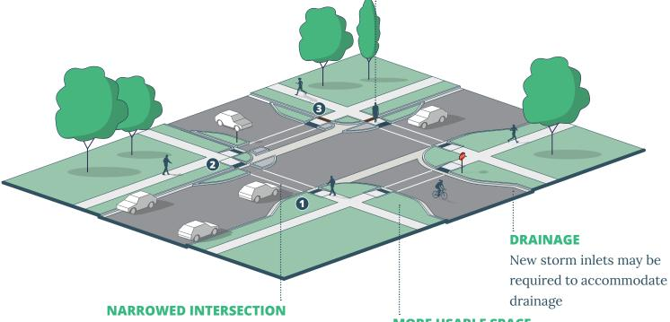
A narrowed intersection creates a shorter crossing distance for pedestrians and causes drivers to slow down through the intersection
